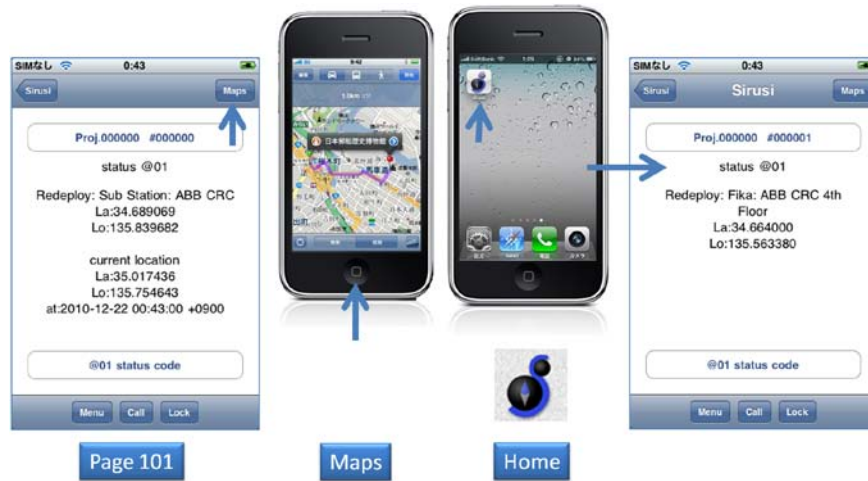
Fig. 3. Smartphone application for locating worksites and managing work orders. Work orders describe repair and maintenance activities step by step, which are updated in real-time by activity recognition methods. In addition, conventional navigation aids for finding the worksite are embedded in the application.
