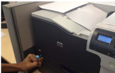
Figure 11: Activity sensing application of ubicuts that create an activity stream entry from the printer's logo every time the user reaches for newly printed papers.
